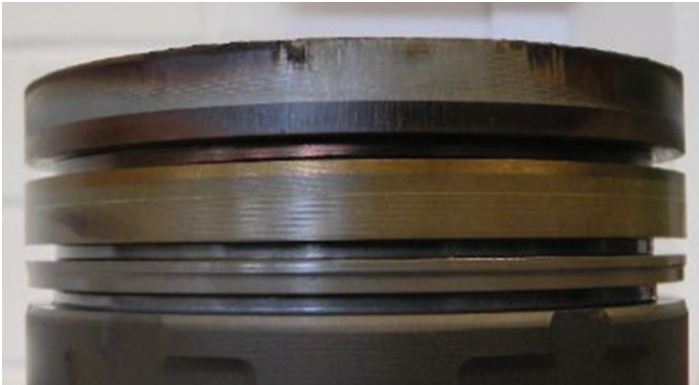
WMM TCG 2016 piston at end of Approval Test showing minimal deposit formation (9,644 hours)
