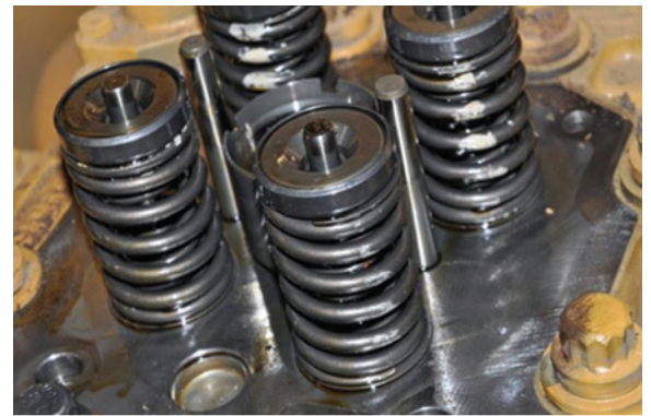
Caterpillar G3516 TALE E+ valve springs at end of Approval Test (8,089 hours)
