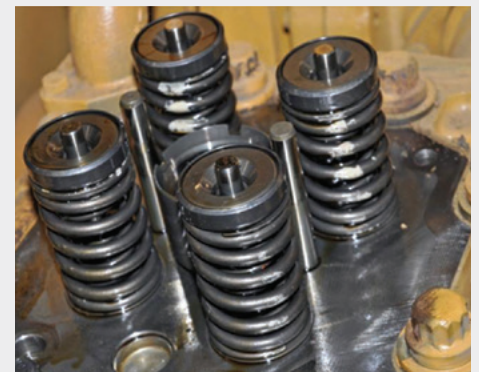
Caterpillar G3516 TALE E+ valve springs at end of Approval Test (8,089 hours)
