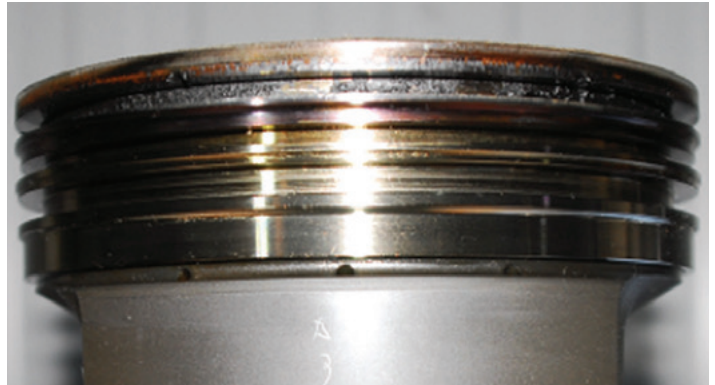
GE Jenbacher 6F piston at end of Approval Test (8,839 hours)
