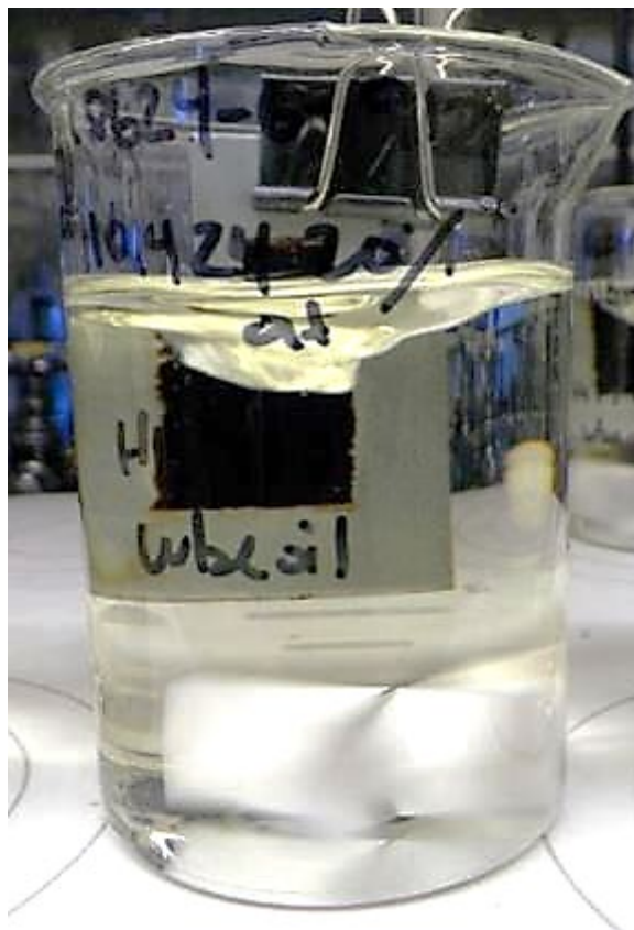
Cleaning Test Apparatus
