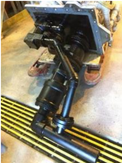
Picture of seized aux oil pump after cleaning with competitor product in 2017
